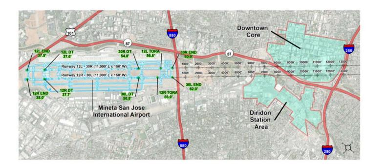
The two normal-flow arrival flight paths correspond to the two black lines extending beyond each of the two SJC runways, and showing the distance in feet from the end of each runway (30R and 30L).
